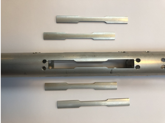
Fig. 5. An illustration of how tensile specimens are cut from the tested tube at different circumferential positions.
