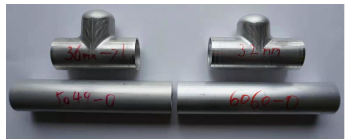
Fig. 11. Hydro bulged specimens before and after test for aluminium alloy 5049-O and 6060-O.
