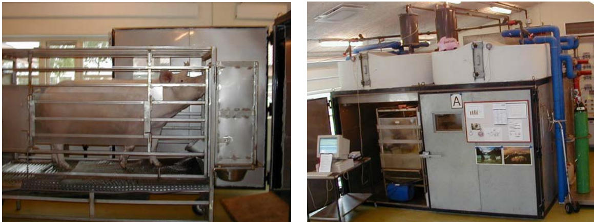
Figure 4.6.2 - A sow in a metabolic cage in the respiration chamber. Photos: Henry Jørgensen.
