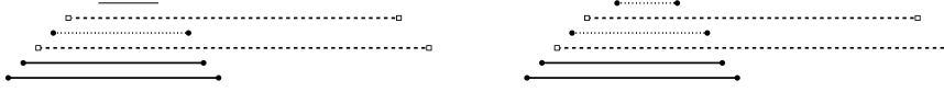
Fig. 5: One iteration of the for loop of Algorithm Online is illustrated here ( h = 2 ). To the left a new interval arrives (at the top with no endpoint symbols). The set \mathcal{H} consists of two chains. To the right we see the new interval joining the chain with black circles as endpoints. The new interval receives the same color as the interval below it in that chain.
