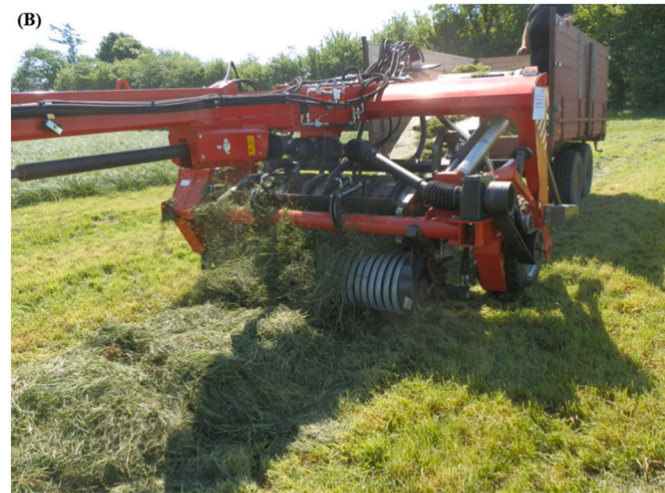
Fig. 1. Schematic diagram of the machine for shredding viewed from the side, where the curved arrows represent the flow of grass-clover (A; diagram by P. Waldemar), and a picture of the shredder prototype in operation (B; picture by M. R. Weisbjerg).
