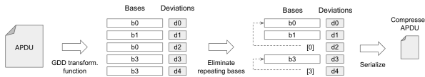
Fig. 2: Compressing each APDU as an independent block. Chunks are transformed to pairs of bases and deviations, and repeating bases are replaced by a base index.
