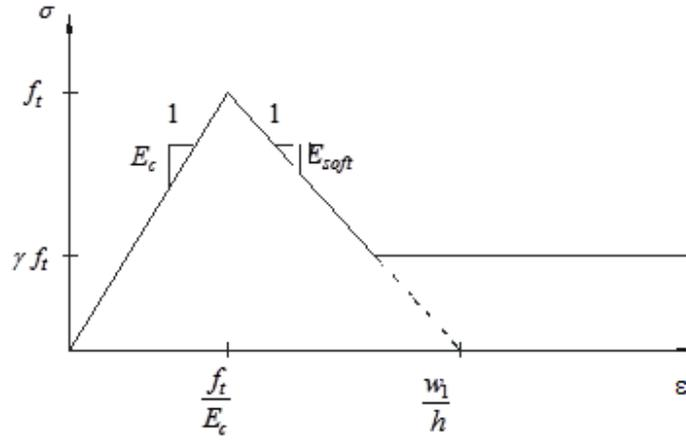
**Fig. 2** Stress strain relation of the fracture band.
