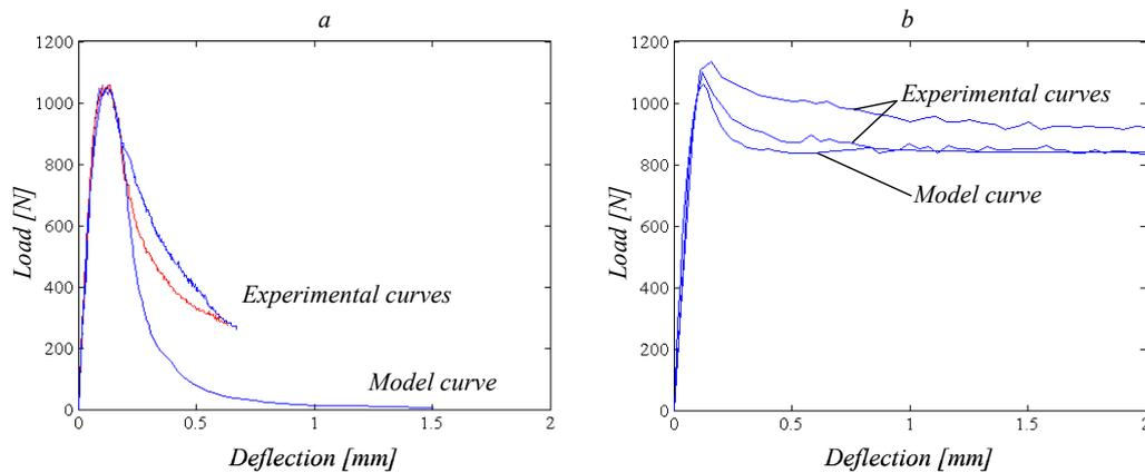
**Fig. 10** Measured and model result for load deflection curves for notched beams of NSC. Left: Concrete without fibers. Right: Concrete with 1.0 VOL% steel fibers.
