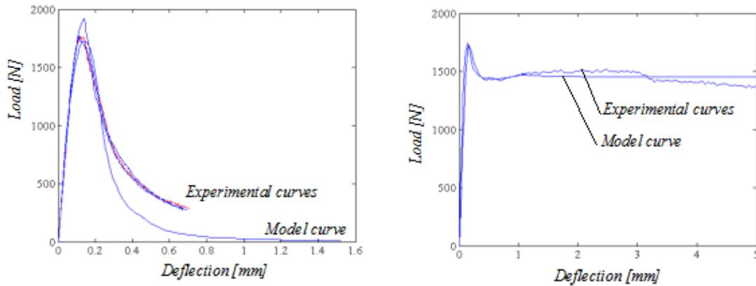
**Fig. 11** Measured and model result for load deflection curves for notched beams of NSC. Left: Concrete without fibers. Right: Concrete with 1.0 VOL% steel fibers.
