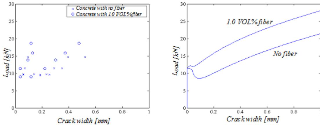
Fig. 18 Left: crack width measurements for NSC 200x400x4800 mm beam with main reinforcement ratio of 0.25 %. Right: Crack widths obtained from the model.
