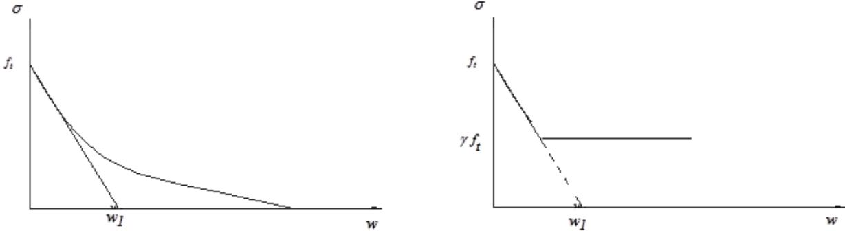
Fig. 1 Stress crack width relation for FRC.
