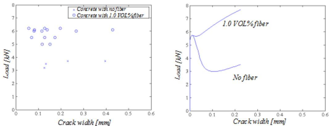
**Fig. 14** Left: crack width measurements for HSC 100x200x2400 mm beam with main reinforcement ratio of 0.14 %. Right: Crack widths obtained from the model.
