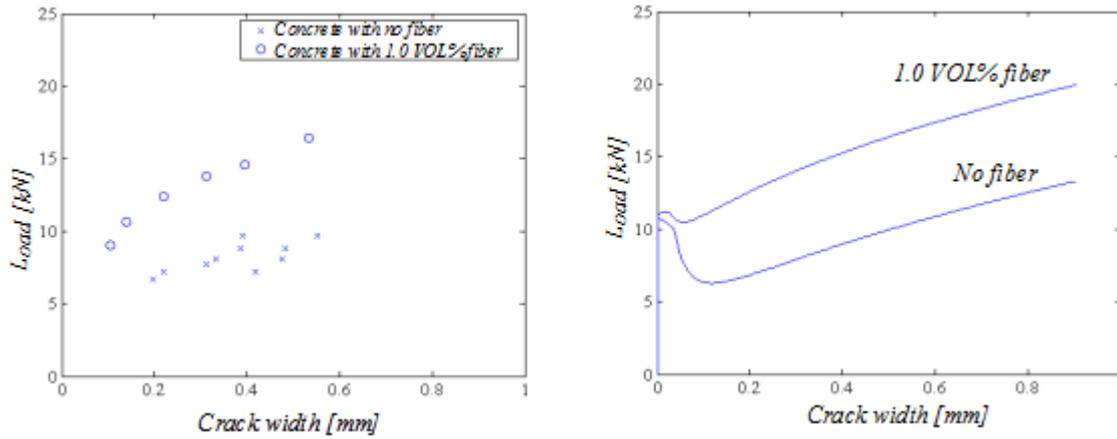
Fig. 17 Left: crack width measurements for NSC 200x400x4800 mm beam with main reinforcement ratio of 0.14 %. Right: Crack widths obtained from the model.
