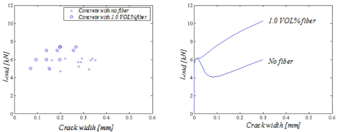
**Fig. 16** Left: crack width measurements for HSC 100x200x2400 mm beam with main reinforcement ratio of 0.25 %. Right: Crack widths obtained from the model.
