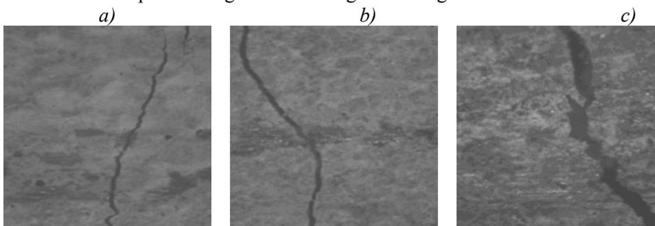
**Fig. 12** Images from crack width measurements. The cracks shown here are measured to a) 0.08 mm. b) 0.12 mm. c) 0.31 mm.
