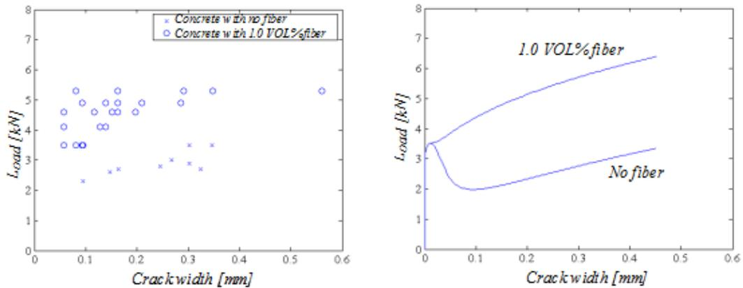
**Fig. 13** Left: crack width measurements for NSC 100x200x2400 mm beam with main reinforcement ratio of 0.14 %. Right: Crack widths obtained from the model.
