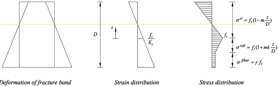
**Fig. 3** Basic assumptions concerning the kinematics of the fracture band and the corresponding stress distribution.
