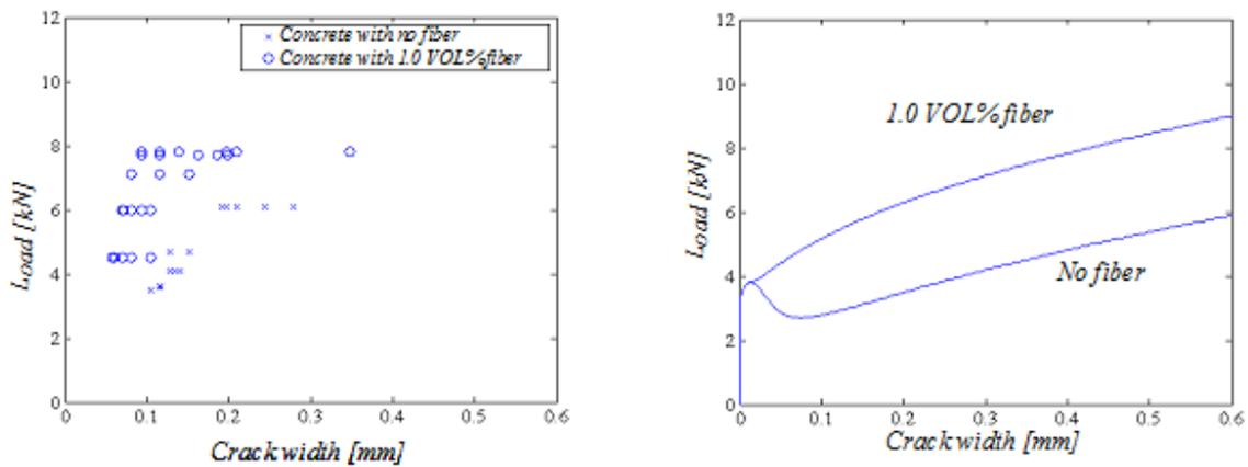
**Fig. 15** Left: crack width measurements for NSC 100x200x2400 mm beam with main reinforcement ratio of 0.25 %. Right: Crack widths obtained from the model.
