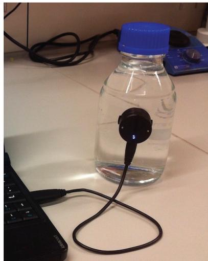
**Fig 1. Device Configuration.** A representation of the LUMOS readout device (left) and its application for measurements in a glass bottle (right). The LUMOS casing features small notches that can be used as attachment points for mechanical mounting of the device to a vessel wall. The flat front surface is also very well suited for using adhesive tape for mounting.
