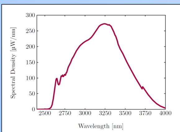
Fig. 2: Supercontinuum spectrum in the MIR region from the ZBLAN fiber output.
