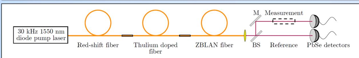
Fig 1: Supercontinuum setup for spectroscopic analysis in the MIR region
