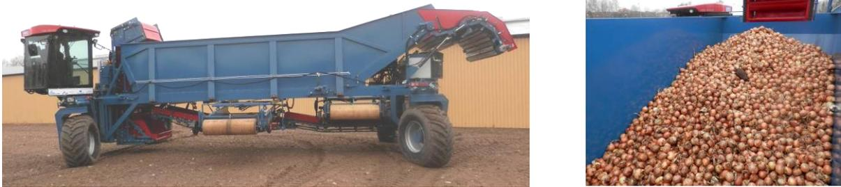
Fig. 3: The wide span tractor mounted with an onion bunker harvester. Photos: Rasmus Meyer, ASA-Lift A/S
