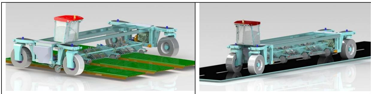
Fig. 3: Conceptual design of a wide span tractor. Left in position for field operations. Right in position for road transport. Drawings: ASA-Lift A/S
