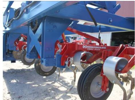
Fig. 1: First test of the wide span tractor, June 2012. The tractor has three 3-point linkages shown here with three Kongskilde cultivators.
