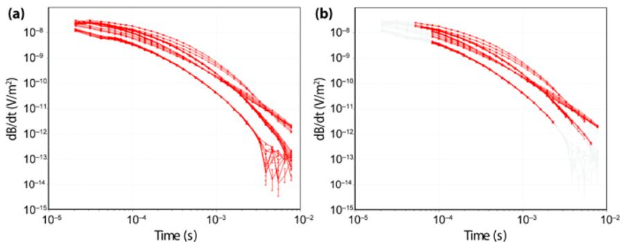
Figure 1. Editing of time gates for 25 example recordings. (a) No editing showing all 33 time gates from 21 - 7828  $\mu\text{s}$  for all recordings. (b) The same recordings after gate editing. Early and late time gates were automatically evaluated for anomalous changes in  $\text{dB}/\text{dt}$  that resulted from the effects of residual transmitter current and the onset of significant noise, respectively. Once identified, the affected time gates were eliminated from the processing flow.
