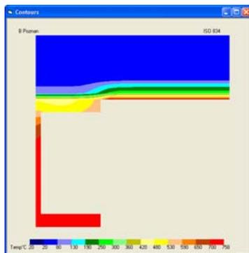
Fig. 2 Half-I-Beam with no shadow effect.
