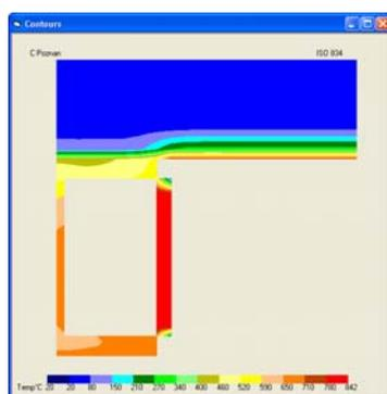
Fig. 3 Half-I-Beam with shadow effect.
