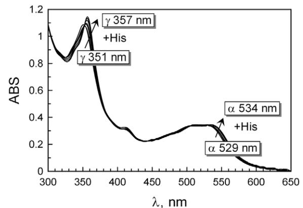
**Figure 5. Absorbance Spectra of Cobalamin bound to Purified Zebrafish Cobalamin Binder.** Spectral characteristics of the zebrafish cobalamin binder in complex with hydroxo-cobalamin are shown. Spectral transition after addition of 15 mM histidine was recorded after 1, 3, 5, 12, 20, and 30 minutes of incubation at room temperature. The arrows indicate the direction of this transition. doi:10.1371/journal.pone.0035660.g005
