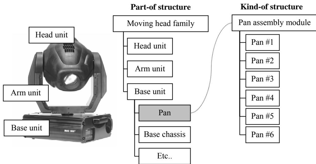
*Figure 2: The product family analyzed in the case is a so-called “moving head”. The base unit consists of several assembly modules. The product family has six different variants of the pan assembly module.*
