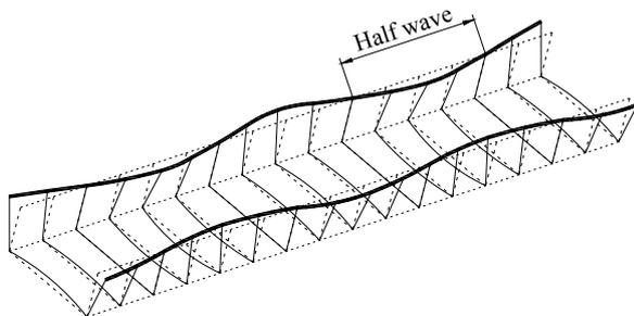
Fig. 2. Buckled shape of girders with U-frames
