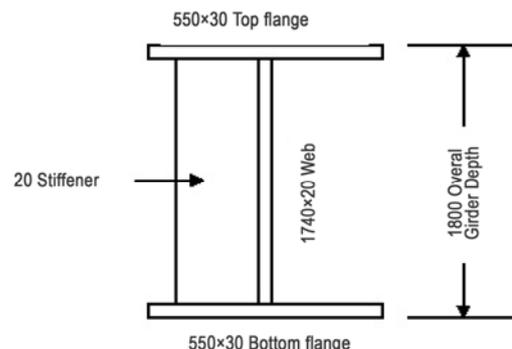
Fig. 3. Cross section of the main girders
