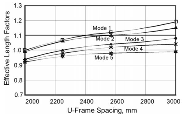
**Fig. 9.** Variation of Effective Length with U-frame spacing
