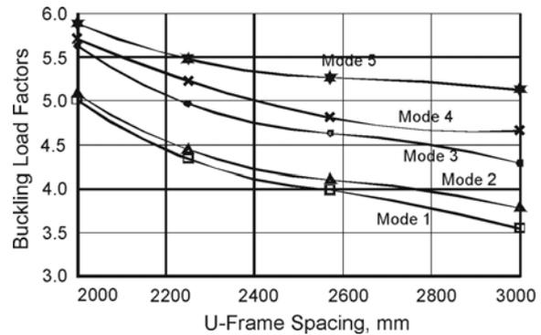
**Fig. 8.** Variation of Buckling Load factor with U-frame spacing
