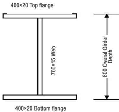
Fig. 4. Cross section of the transverse girders
