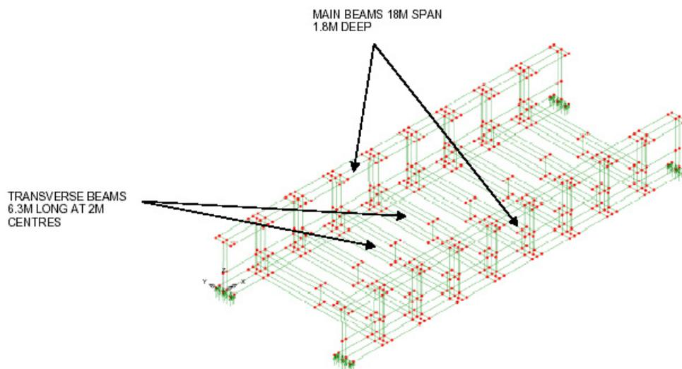
Fig. 5. FE model of girders with U-frames
