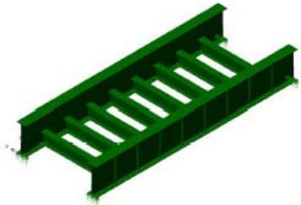
Fig. 1. Typical girders with U-frame
