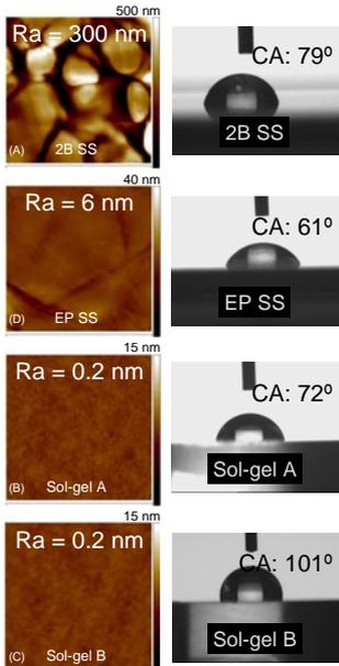
TappingMode AFM height images. Height scale 15-500 nm. A: scan size 10 x 10 µm<sup>2</sup>. B-D: Scan size 2 x 2 µm<sup>2</sup>
