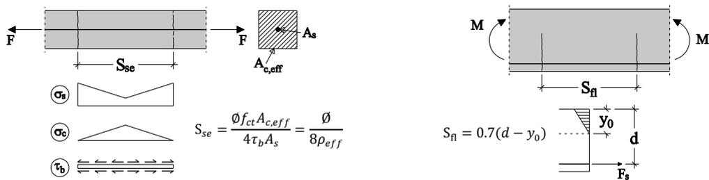
Fig. 3. (a) Tension Chord Model for crack spacing; (b) Estimation of crack spacing in flexural members by Reineck.
