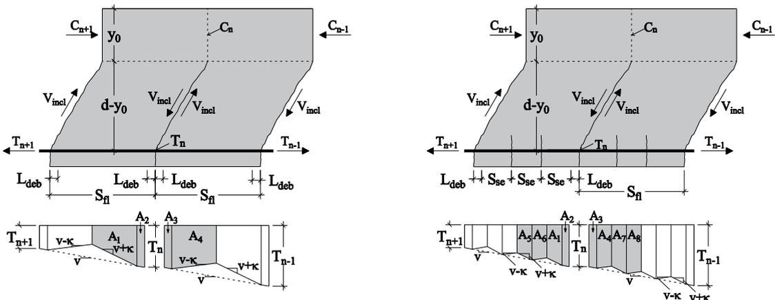
Fig. 5. Forces within three flexural cracks (a) only flexural cracks occurring; (b) both flexural and secondary crack occurring.
