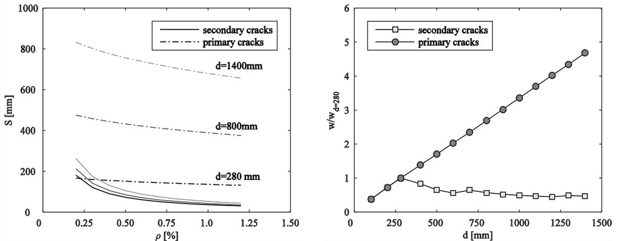
Fig. 7. (a): Relations between relative crack spacing and reinforcement ratio, for effective depths of  $d=280\text{mm}$ ,  $d=800\text{mm}$  and  $d=1400\text{mm}$
