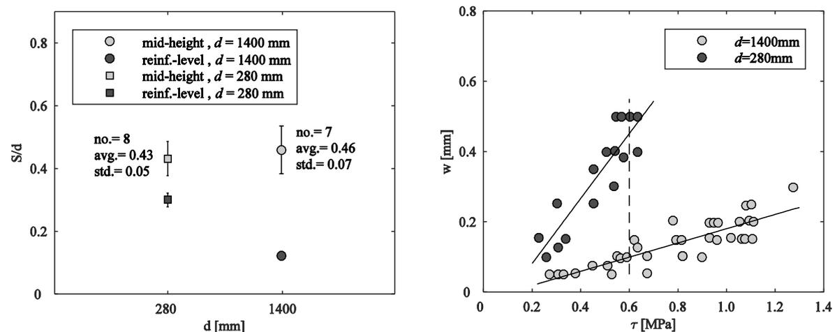
Fig. 2. Test by Sherwood (a) average crack spacing for complete test series; (b) measured crack widths in small and large beams.
