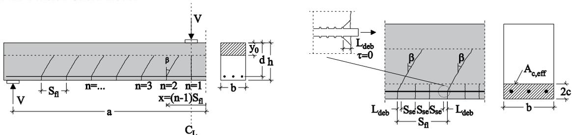
Fig. 4. (a) Assumed flexural crack pattern; (b) Assumed crack pattern of secondary cracks in fictitious tension bar and debonded zone.
