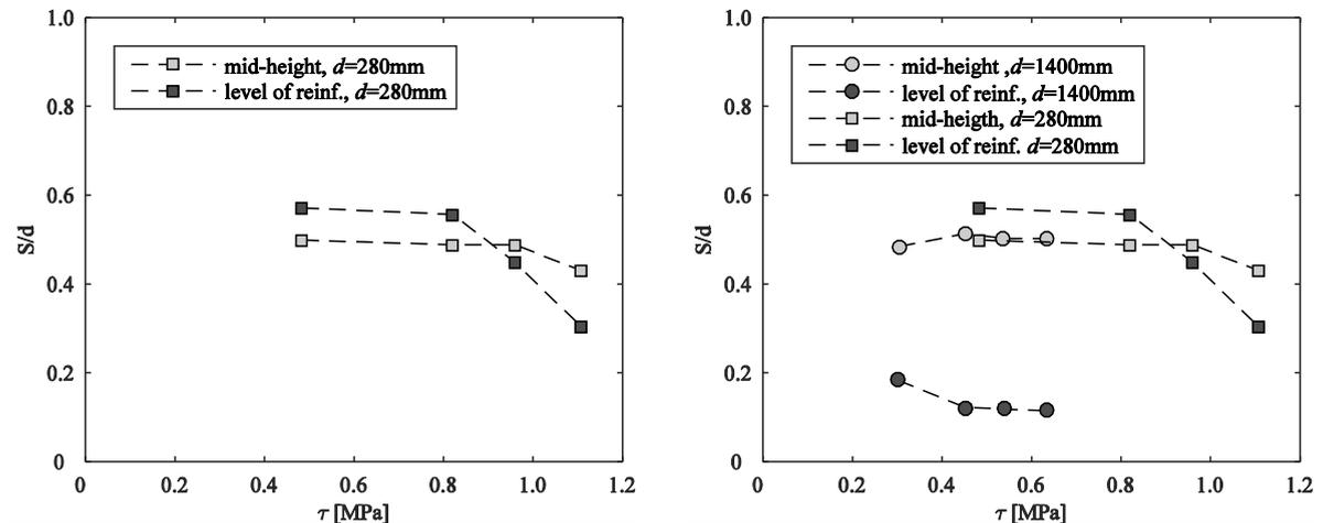
Fig. 1. Tests by Sherwood (a) relative crack spacing for small beam; (b) for large and small beam.
