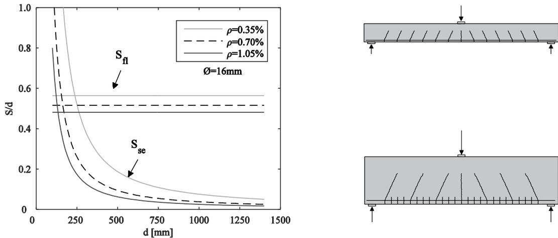
Fig. 6. Relations between relative crack spacing and effective depth, for reinforcement ratios;  $\rho=0.35\%$ ,  $\rho=0.7\%$  and  $\rho=1.05\%$ .
