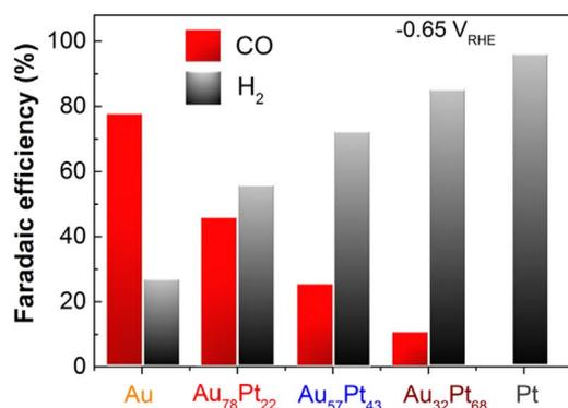
Fig. 2. Faradaic efficiency for CO on Au-Pt bimetallic alloys with different compositions at -0.65 V versus RHE in CO<sub>2</sub>-saturated 0.1 M KHCO<sub>3</sub> electrolyte (pH = 6.8).
