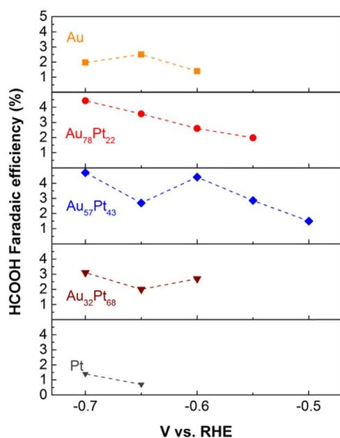
Fig. 4. Faradaic efficiency for HCOOH formation at various potentials in CO<sub>2</sub>-saturated 0.1 M KHCO<sub>3</sub> electrolyte.
