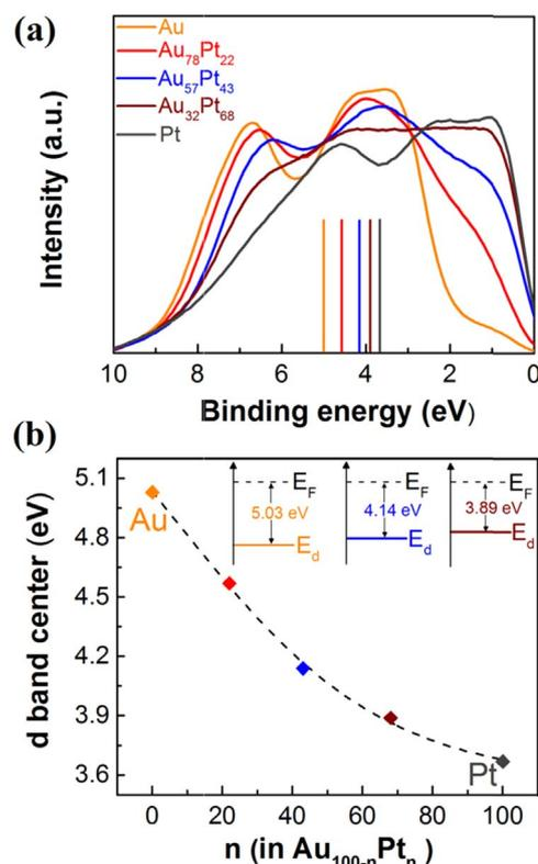
Fig. 5. Electronic properties of Au-Pt bimetallic films. (a) Comparison of surface valence band XPS spectra of Au-Pt bimetallic films with different composition (the binding energy is the value of  $|E-E_F|$ ). The color line in the center represents the position of d-band center of the corresponding Au-Pt film. (b) Energy of d-band center as a function of Pt content. The inset shows the d-band center ( $E_d$ ) position of Au and Au-Pt alloys with respect to the Fermi level.
