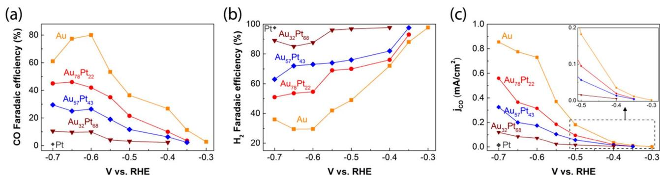
Fig. 3. Comparison of the electrocatalytic performance of Au-Pt bimetallic alloys with different compositions. Faradaic efficiency for CO (a) and H<sub>2</sub> (b) on Au-Pt bimetallic alloys with different compositions at various potentials in CO<sub>2</sub>-saturated 0.1 M KHCO<sub>3</sub> electrolyte (pH = 6.8). (c) Partial current density for CO at various potentials.
