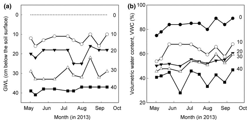
**Fig. 2** Dynamics of (a) measured groundwater level (GWL) and (b) volumetric water content at the five nominal GWL during the study period from May to September 2013. Numbers next to lines indicate the different GWL treatments (cm below soil surface); dotted line indicates that water was always visible at the surface of the 0 cm GWL treatment. Volumetric water content was measured at 0–5 cm depth for 0 cm GWL, at 0–10 cm depth for 10 cm GWL and at 0–20 cm depth for 20, 30 and 40 cm GWL.
