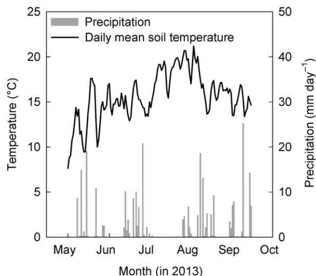
**Fig. 1** Daily precipitation and mean daily soil temperature at 5 cm depth in the mesocosms. Data represent all five groundwater-level treatments during the study period from May to September 2013.
