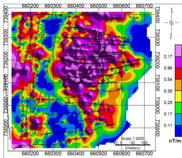
**Figure 2:** Map of the magnetic analytical signal showing the position of waste with high magnetic signature. Black hollow circles represent the acquisition points.
