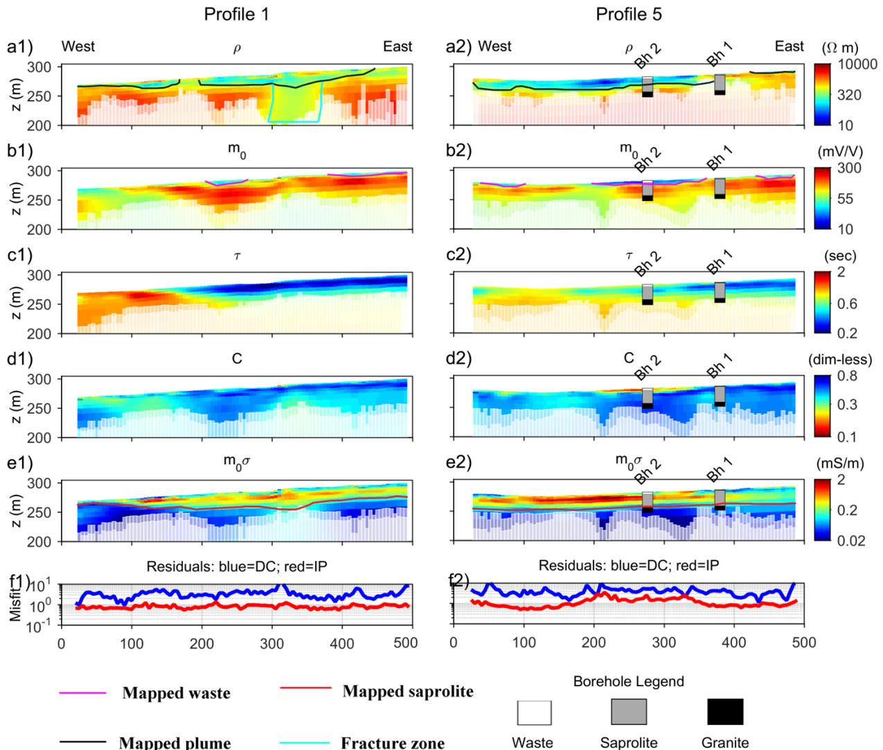
Figure 3: Cole-Cole DCIP parameters of profiles 1 and 5 a) resistivity section showing the picked plume bottom and fracture zone b) chargeability section showing the waste bottom c) relaxation time section d) frequency factor section e) normalized
