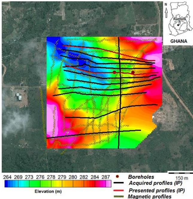
**Figure 1:** Satellite image of the study area showing the acquired profiles (black and red lines), the borehole positions (dark red circles), the magnetic lines (dark green cross) and the digital elevation map.
