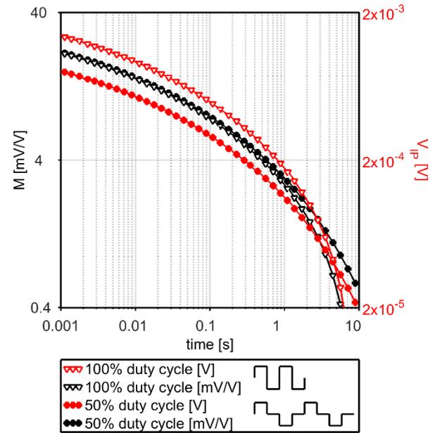
**Figure 3.** 50% duty cycle decays (circles) and 100% duty cycle decays (triangles) for Cole-Cole homogeneous halfspace ( $\rho=100$   $\Omega$ m,  $m_0=40$  mV/V,  $\tau=0.01$  s,  $C=0.3$ ,  $T_{on}/T_{off}=10$  s, 4 stacked pulses). Black lines represent the normalized decays in mV/V, while red lines represent the actual voltages (see Olsson *et al.* (2015) for details).
