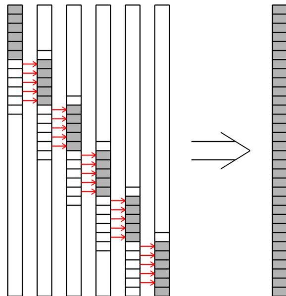
**Figure 4.** Split of a 32-layers 1D model (grey model) in six 13-layers laterally-constrained sub-models for computational efficiency. The red arrows represent the lateral constraints.
