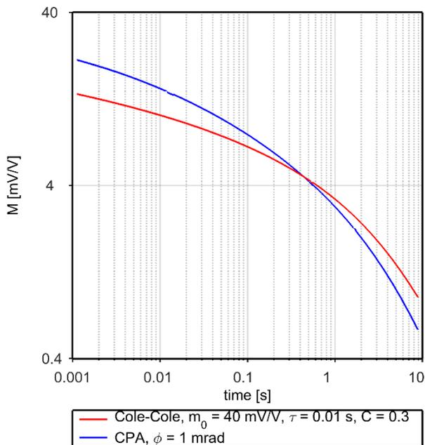
**Figure 2.** Examples of Cole-Cole decay (red curve) and CPA decay (blue curve) for homogeneous half spaces and 50% duty cycle waveform ( $T_{on} = T_{off} = 10$  s, 4 stacked pulses).
