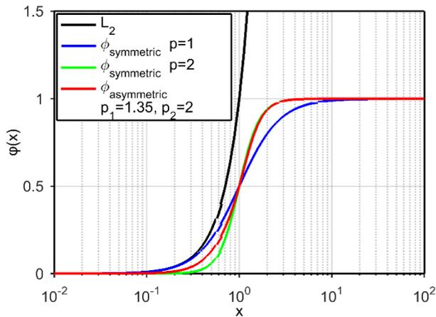
**Figure 5.** Comparison of  $L_2$  norm, symmetric minimum support (equation 4) and asymmetric minimum support (equation 5) with varying norm settings.
