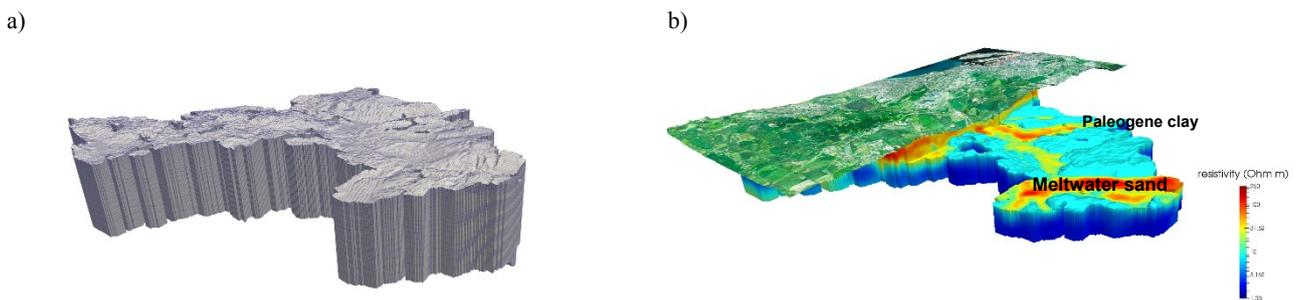
**Figure 1. Voxel inversion. a) shows the voxel grid with a 30 layer vertical discretization and 40mx40m cells. b) shows a cut into the resulting resistivity model after inversion.**
