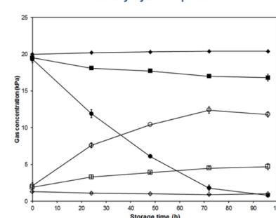
Fig 1. O<sub>2</sub>/CO<sub>2</sub> gas concentrations inside packages with wild rocket Control (◆/◇); high OTR at 20 °C (■/□); low OTR at 20 °C (●/○).
