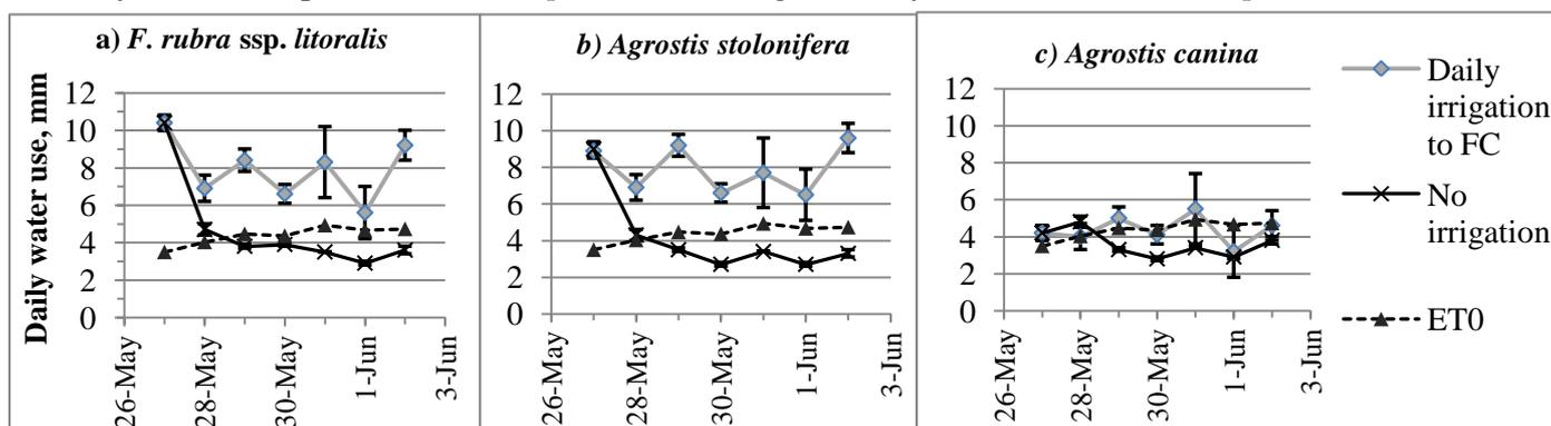
Fig. 1. Effect of daily irrigation to field capacity vs. no irrigation on daily water consumption of three turfgrass species on a USGA green from 27 May to 2 June 2009. Reference  $ET_0$  is also indicated.
