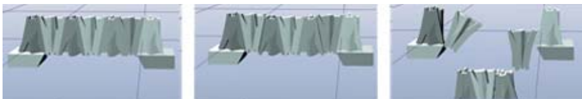
Figure 11: Displacement of the interlocking blocks of Fig.7, assuming frictionless contacts, at simulation time t equal 0s, 0.1s and 0.5s.
