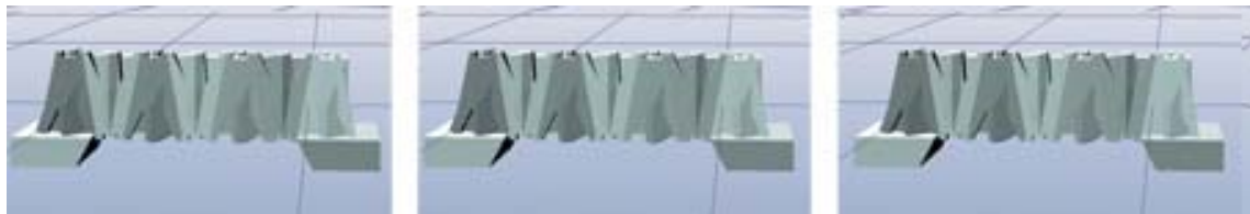
Figure 10: Displacement of the interlocking blocks of Fig.9 at simulation time t equal to 0.5s, 2s and 3s
