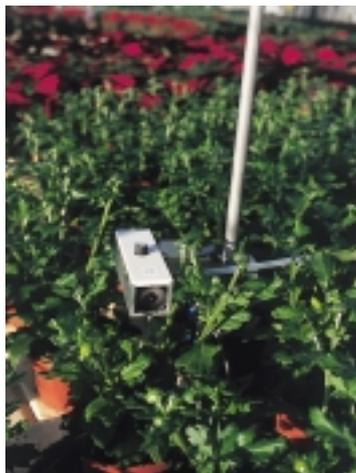
A series of sensors is coupled to a small ventilated box where air and leaf temperature, irradiance, CO<sub>2</sub> concentration and air humidity are measured in the vegetation.
