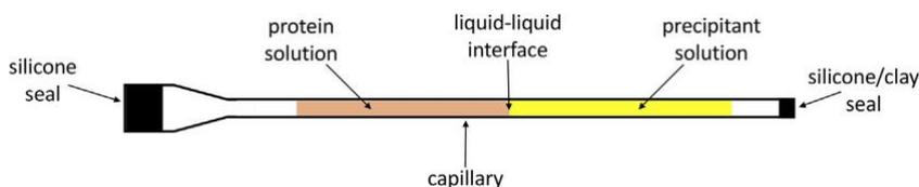
**Fig. 5** Schematic of the capillary counterdiffusion format. First protein, then an equal volume of precipitant solution is carefully aspirated into a capillary (such that the two liquids are touching). Both ends of the capillary are then sealed with silicone sealant/clay and the entire setup moved into a temperature-controlled environment to incubate.
