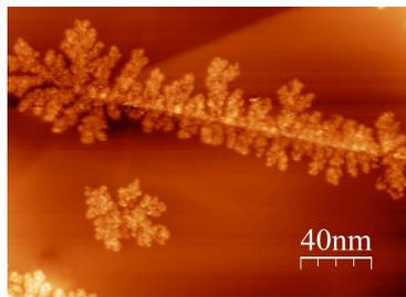
Figure 1: LT-STM image of water ice clusters on HOPG (4.5 V, 15 pA)
