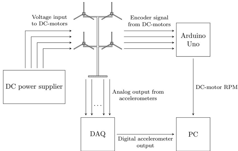
**Figure 4.** Flowchart of the data acquisition system.
