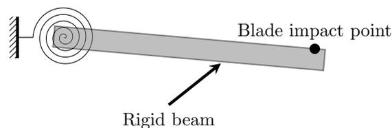
**Figure 3.** Automated blade impact mechanism used to excite blade modes.
