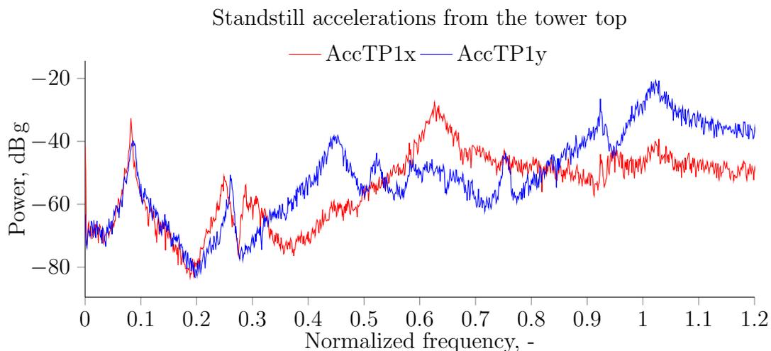
**Figure 5.** Power spectral density plot from standstill analysis from the two accelerometers on the tower top.
