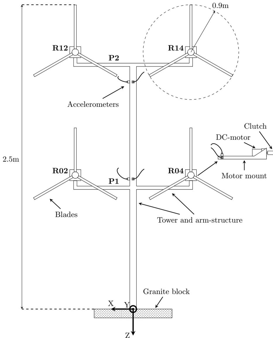
**Figure 2.** Illustration of the main components of the scaled experimental setup of the Vestas four-rotor wind turbine. R02, R04, R12 and R14 refers to the different rotors. P1 refers to the lower platform, and P2 to the upper platform.
