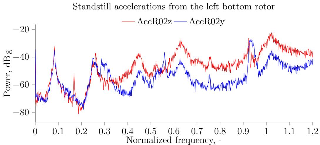
**Figure 6.** Power spectral density plot based on acceleration data from nacelle R02 at standstill.
