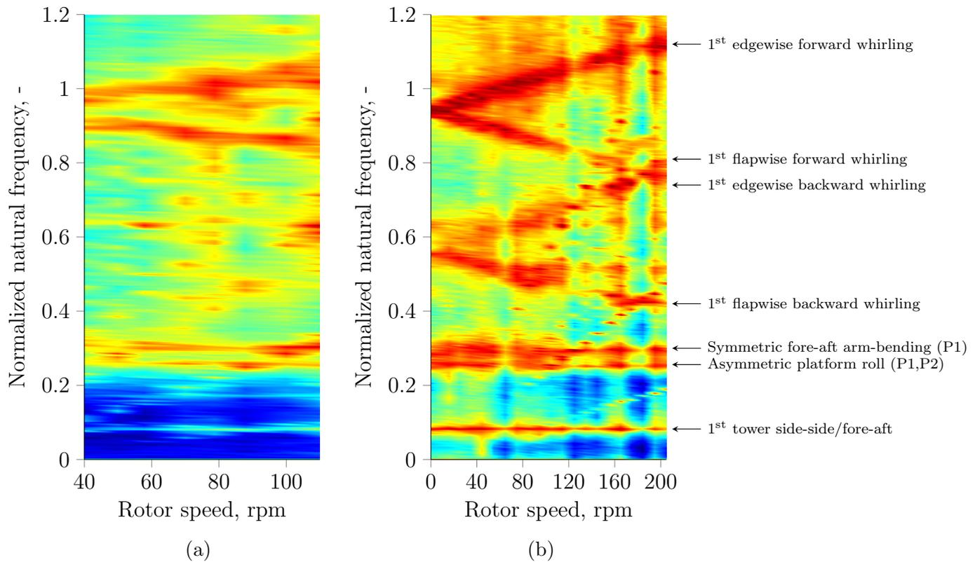
**Figure 7.** Campbell diagrams for the experimental setup based on the automated impulse mechanism from 40 to 110 rpm (a), and using the metal brushing technique from 0 rpm to 205 rpm (b). Both diagrams used acceleration data from rotor R02 in global z direction.
