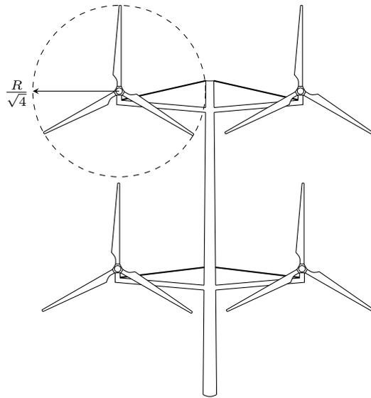
**Figure 1.** Illustration of Vestas four-rotor concept demonstrator. Tip height was 75 m, and it had four 27 m rotors.  $R$  refers to the radius for a single-rotor wind turbine with the equivalent power output.
