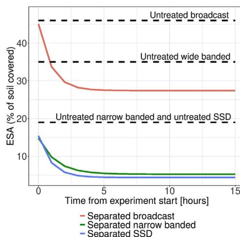
**Fig. 3 – Exposed surface area after field application of 60 metric ton ha<sup>-1</sup> separated and untreated cattle slurry to bluegrass with different application techniques. Narrow banded: as trailing hose application, wide banded: banded in 0.2 m wide line, SSD: narrow band applied over sub-surface deposition aeration slots. Area for untreated slurry is estimated to be constant over time (dashed lines).**
