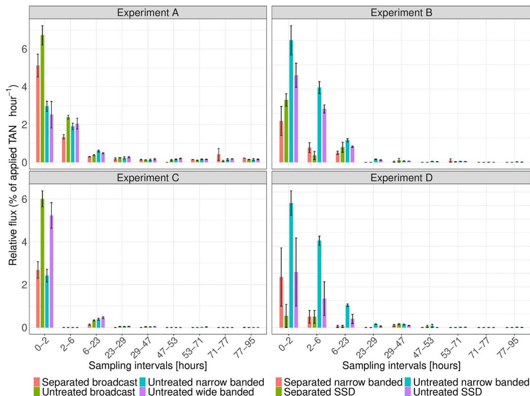
**Fig. 1 – Ammonia flux after application of 60 metric ton ha<sup>-1</sup> untreated and separated cattle slurry to bluegrass with different application techniques. Narrow banded: as trailing hose application, wide banded: banded in 0.2 m wide line, SSD: narrow band applied over sub-surface deposition aeration slots. Standard errors are displayed as vertical error bars (n = 4).**
