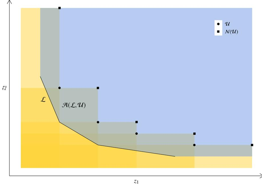
Figure 1: Given a lower bound set  $\mathcal{L}$  (the line segments) and an upper bound set  $\mathcal{U}$ , the search region  $\mathcal{A}(\mathcal{L}, \mathcal{U})$  is given by the closure of the gray area.
