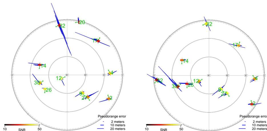
**Fig. 2.** Skyplots of measurements at two locations inside the warehouse.
