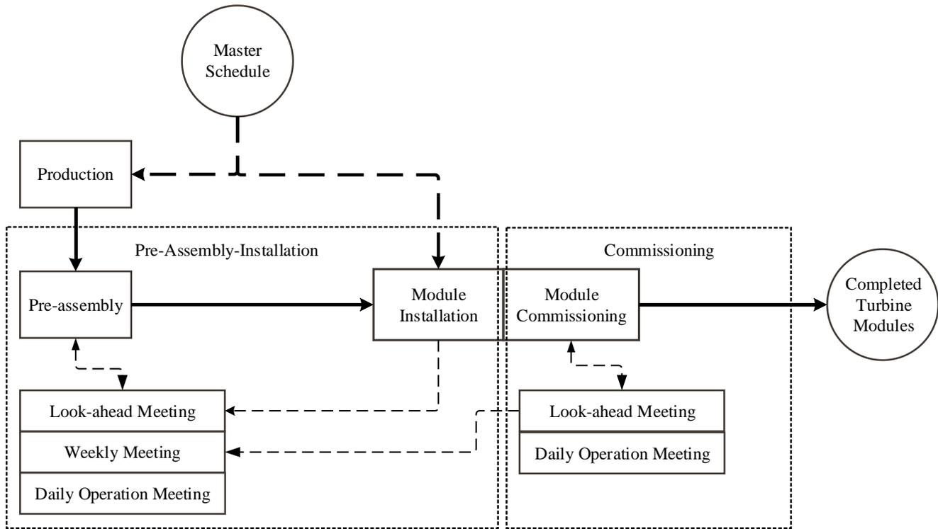
Figure 31: Modular offshore wind construction LPS model (Lerche et al., 2020a)
