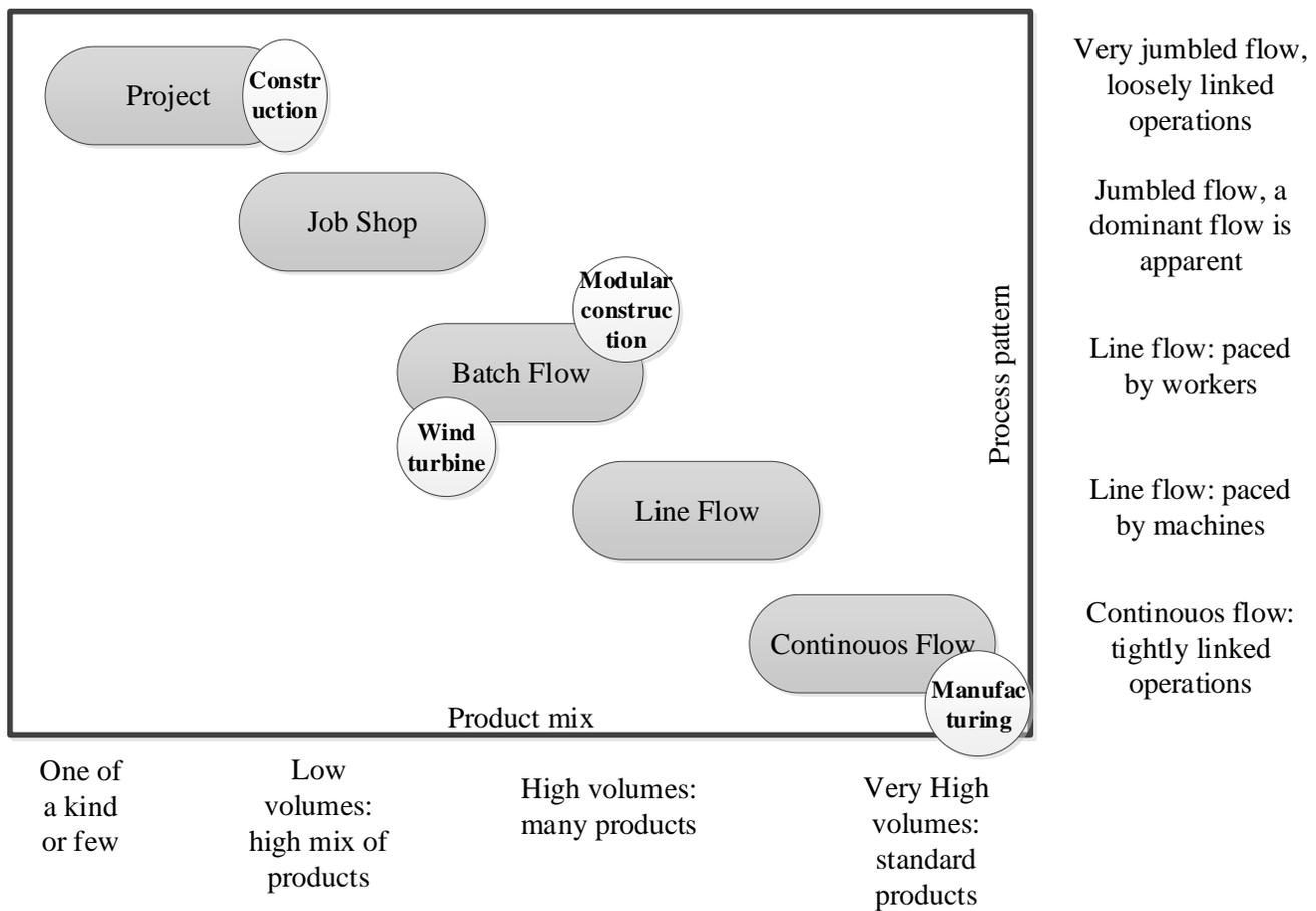
Figure 4: Comparing modular offshore wind construction with manufacturing and construction, modified from (Lerche et al., 2019b).
