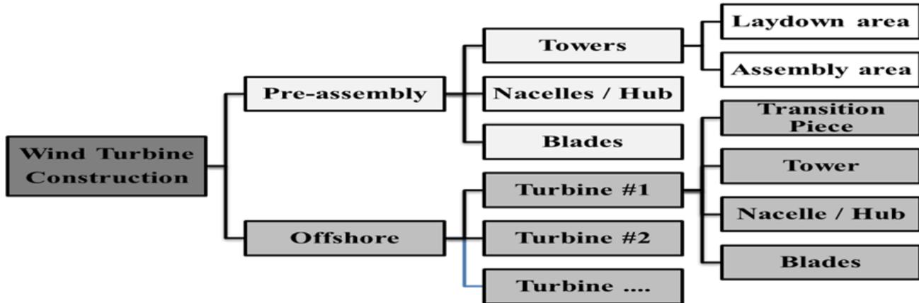
Figure 53: Location breakdown of structure in offshore wind construction (Lerche et al., 2019c).
