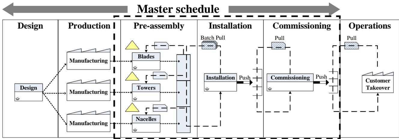
Figure 2: High-level project process map with focus area within dashed square (Lerche et al., 2020a).
