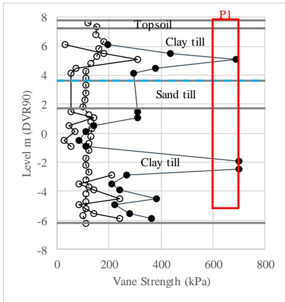
Figure 2. Ground conditions for P1.
