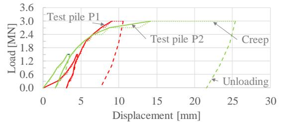
Figure 6. Load-displacement curves for static compression pile load tests on P1 and P2, digitized cf. (Bartsch, 2018).
