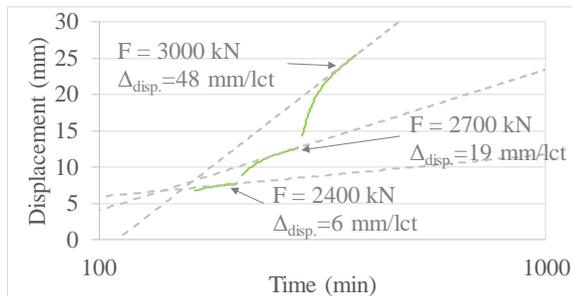
Figure 7. Time-displacement curves for the three last load steps of static compression pile load test P2, digitized cf. (Bartsch, 2018).
