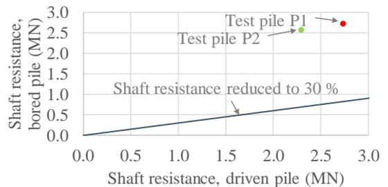
Figure 8. Shaft resistance for bored vs. driven piles.
