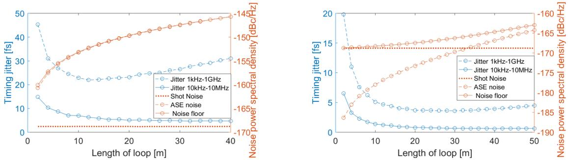
Figure 4. Timing jitter (in fs) as a function of delay length (left axis) and the corresponding noise contributions (right axis). The figure to the left is with ASE-parameters from [4] and the right with ASE-parameters from [5]. Note the difference in scale and range of the axes.
