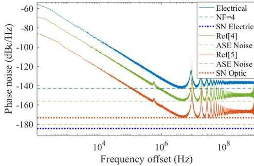
Figure 2. OEO phase-noise simulated with electrical amplifier (blue) and SOA amplifier (green and red). The white noise contributions from shot noise and chosen amplifier are plotted along with the phase noise spectrum. Note that the two simulations with optical amplification share shot noise value.
