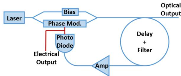
Figure 1. The proposed layout for a PIC based OEO. Note that although no electrical parts are needed in the oscillator loop the laser and amplifier still needs a driving current while the modulator and photo-diode need an applied bias.
