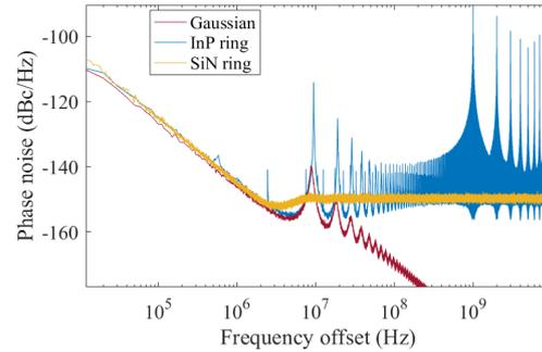
Figure 3. Phase noise spectra of an OEO for varying filter functions and all other parameters equal. The variations are an electrical gauss-passband (red), an InP ring resonator (blue) and a SiN ring resonator (yellow). The spurious peaks are matching with the round-trip time of the OEO.
