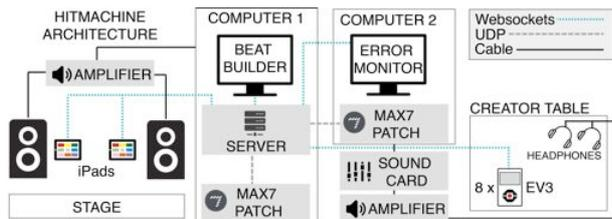
Figure 5. Central components and architecture of Hitmachine.
