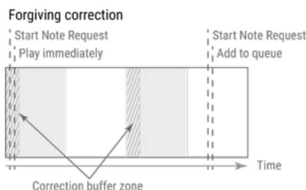
**Figure 11. Forgiving correction. The grey fields are part of the chosen main rhythm and the white are not. If a note is stricken within the timeframe of the crosshatched areas the note will be played immediately instead of queued.**
