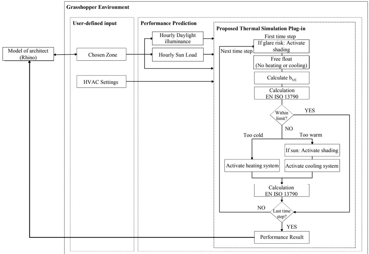
Fig. 1. Schematic of the simulation procedure of the proposed thermal simulation plug-in, and the connection to the sketched 3D-model.
