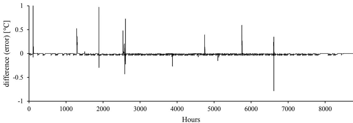
Fig. 3. Hourly differences between the two implementations ( $T_{op,interpolation} - T_{op,analytical}$ ) regarding operative temperature
