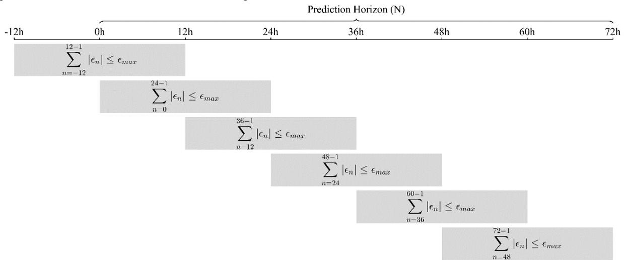
Figure 2. Principle of proposed additional six state constraints
