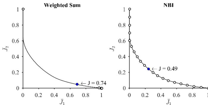
Figure 1. Normalized optimal Pareto solutions with  $\lambda$  increments of 0.05.
