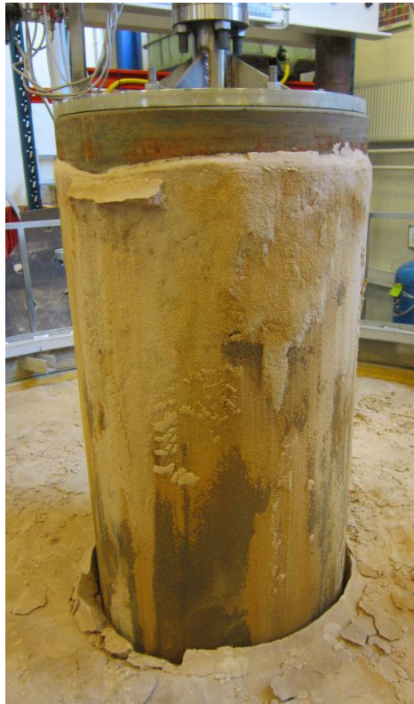
Fig. 5. Uninstallation of the pile after a test with applied suction. Sand is not resaturated before uninstallation, and some sand is stuck to the upper one third of the pile.
