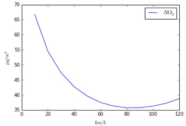
Fig. 9. Modelled  $NO_2$  concentration for different average speeds
