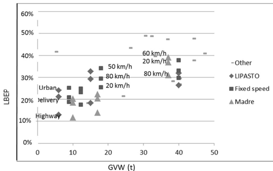
*Figure 4: The effect of driving conditions on the LBEP for fixed speed models and driving conditions according to LIPASTO and Madre et al.*
