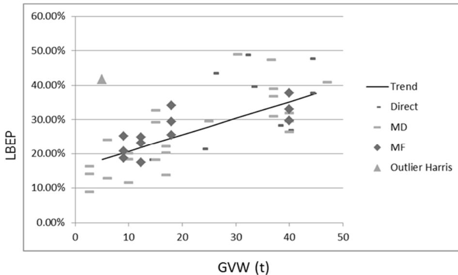
Figure 1: The observations with their LBEP and GVW values and linear regression line, divided into direct observations, models with driving conditions (MD), models with fixed speeds (MF), and the outlier from Harris.
