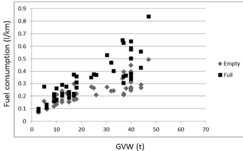
Figure 4: Fuel consumption per km of fully loaded and empty vehicles with GVWs
