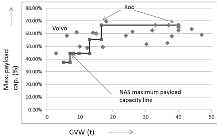
Figure 2: The observed maximum payload capacity as a function of the GVW (points) and the level from the National Academy of Sciences (NAS) from Table 1. Interesting observations are highlighted.
