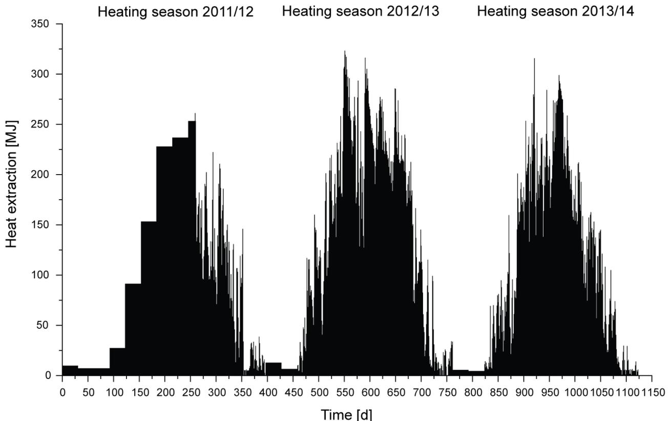
Figure 1. The calculated heat extraction from the ground during the first three years of operation. The first 8 months of heat extraction is estimated.
